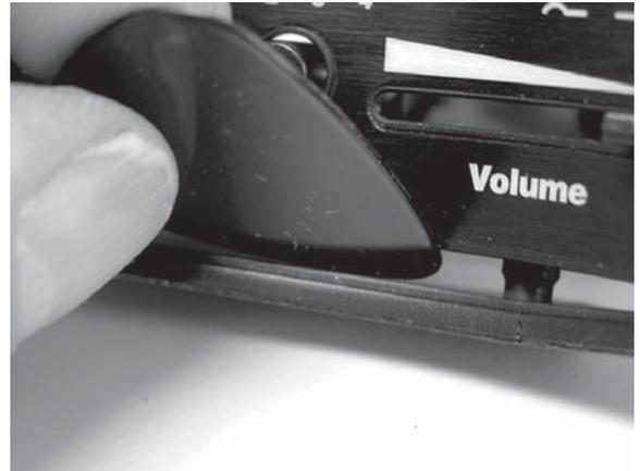
**Figure 3. Separate preamp from bracket**
