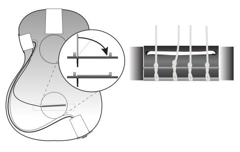
Attach pickup wire (signal wire to IN - shield to GND) battery wire and output jack wire to preamp. Install using four screws and mounting brackets.
