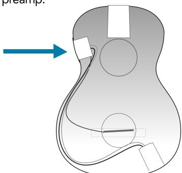
Insert stripped ends of pickup into slot so that when laid flat, the opposite end of pickup lies against slot edge.
